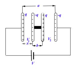
Therefore, potential differences between the pairs of plates are
